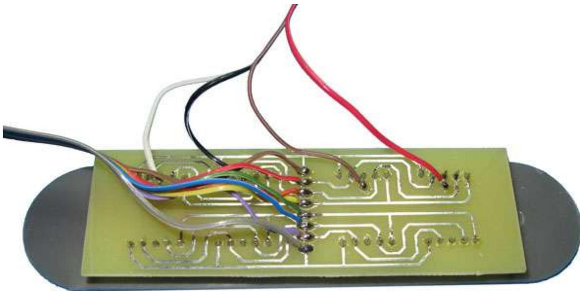
The 8-way cable drives the LED anodes, while the 4-way cable connects each digit's common-cathode to its corresponding driver transistor on the main board.
