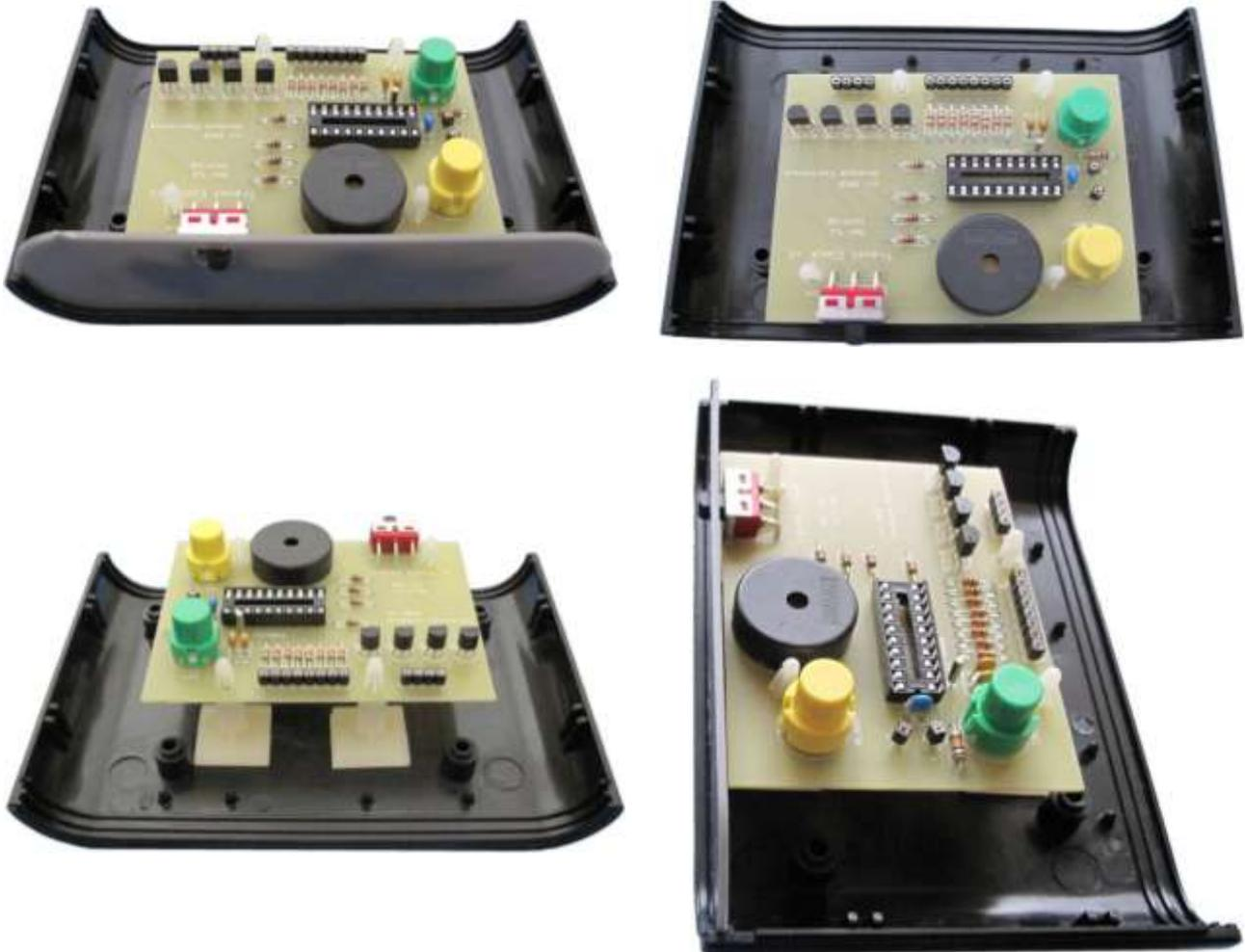
With the PCB supports firmly attached to the base, remove the main board from the supports, and affix the battery holder between the PCB supports, using double-sided tape, as shown.
