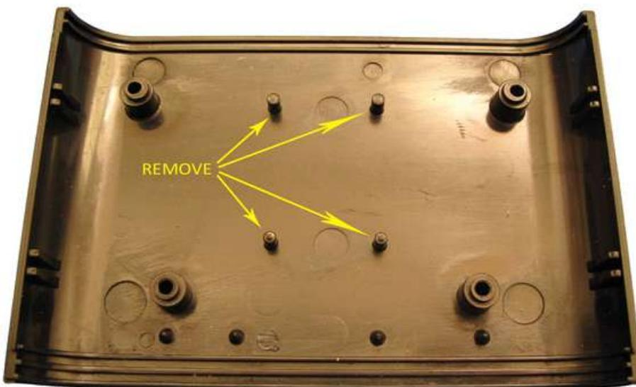
They can be removed using side cutters and then filed flat, or you could use a rotary tool with a cutting wheel attachment.
