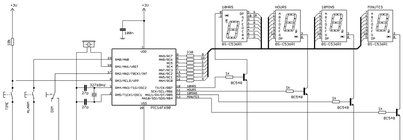
Two AAA batteries provide a nominal 3V power supply. The PIC can operate down to 2.0V, so there is no need for regulation. However, as the battery voltage falls, the display will become dimmer. A "low battery" condition is indicated (by quickly flashing the seconds indicator) when the power supply falls to 2.2 V.
