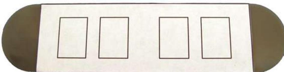
The cut-outs can be made fairly easily by drilling a line of small holes just inside the lines, and then cleaning the edges with a small file.
